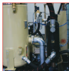
Multi stage separation provides low coolant carry over.
